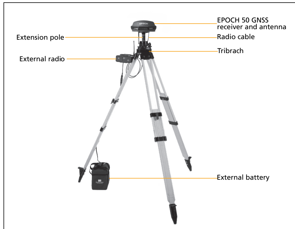
Figure 2.2 EPOCH 50 GNSS receiver, base setup
