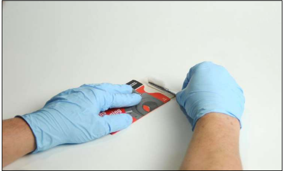
Figure 9-6: Creating a T-shaped cleaning pad (1)
