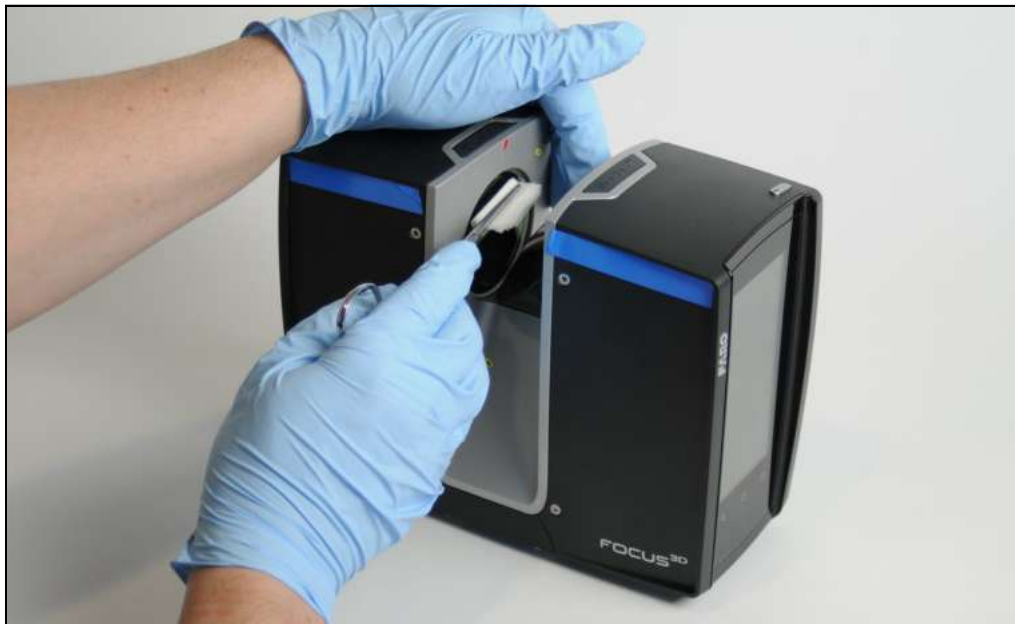
Figure 9-10: Cleaning sensor cover with pad and isopropyl alcohol or cleaning fluid
