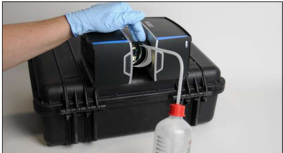
Figure 9-14: Cleaning mirror module or sensor cover
