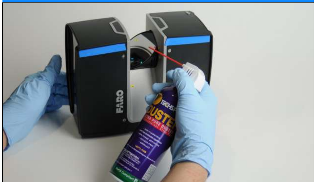
Figure 9-1: Dry pre-cleaning with compressed air or duster cleaning spray
