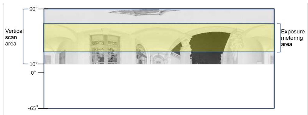
Figure 7-14: Exposure metering area for a limited vertical scan area set to e.g., 10° to 90°
