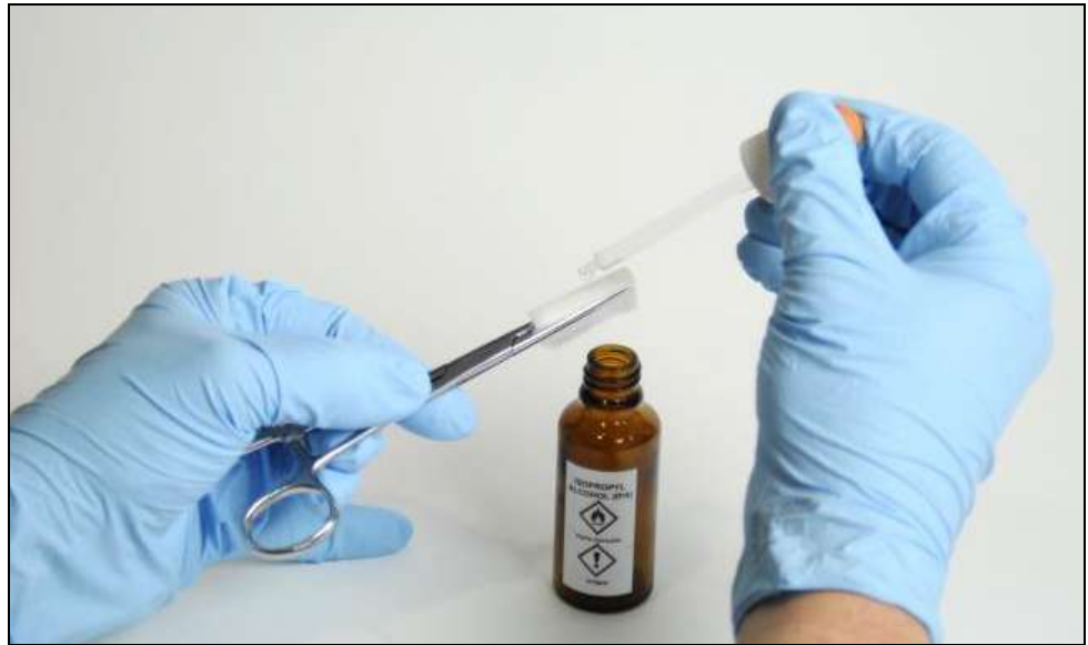
Figure 9-8: Soaking the cleaning pad
