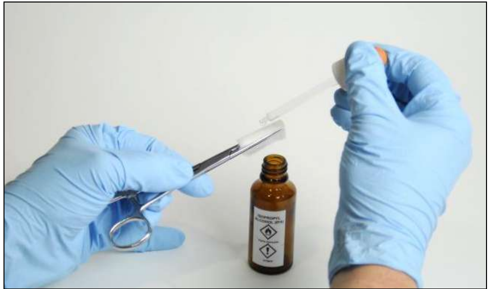
Figure 9-8: Soaking the cleaning pad
