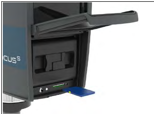
Figure 6-8: Inserting the SD Card
