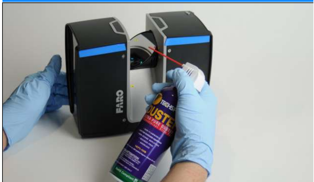
Figure 9-11: Dry pre-cleaning by compressed air or duster cleaning spray
