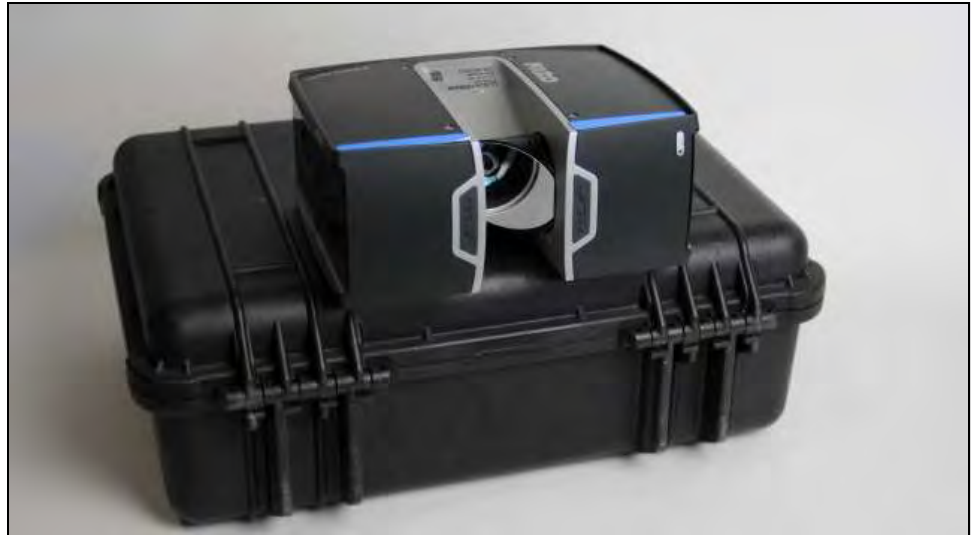
Figure 9-12: Transport box with laser scanner turned and laid on top, with the mirror module facing outwards
