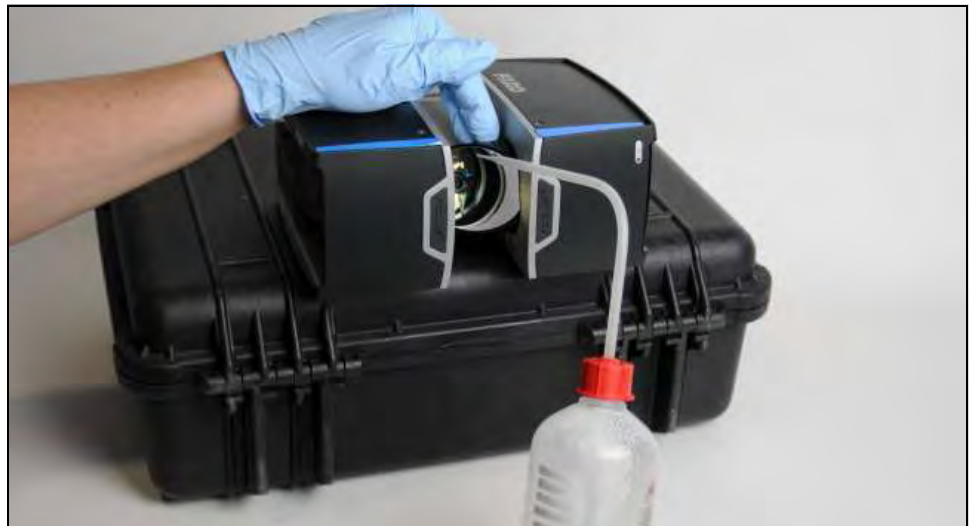
Figure 9-14: Cleaning mirror module or sensor cover
