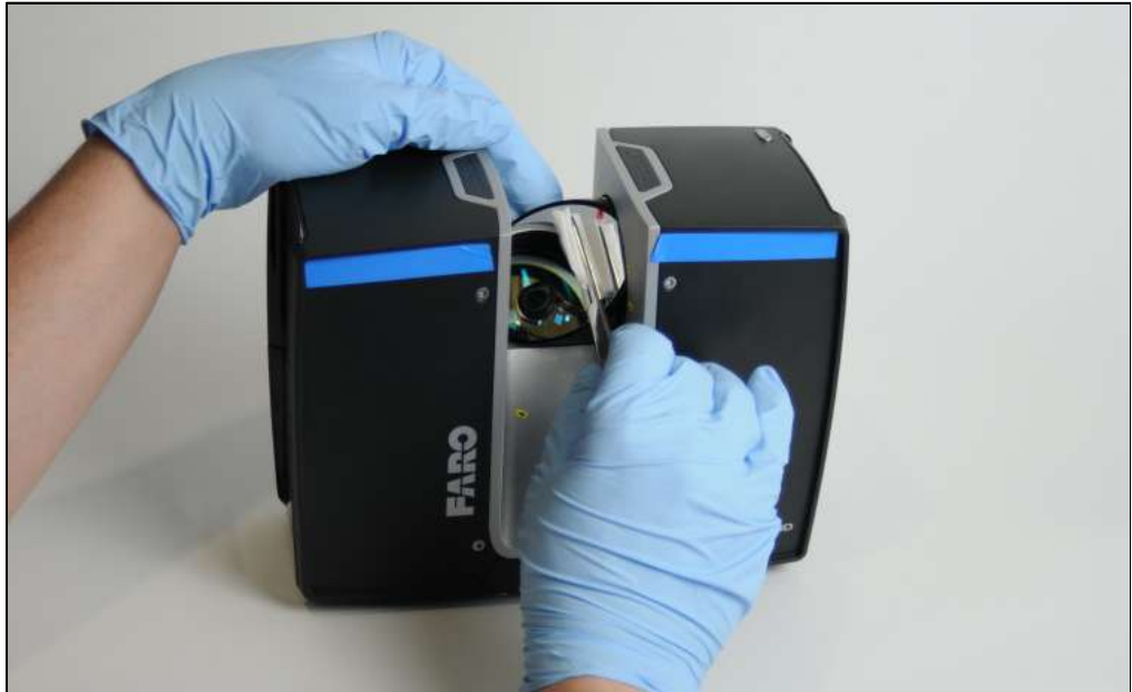
Figure 9-9: Cleaning mirror module with pad and isopropyl alcohol or cleaning fluid
