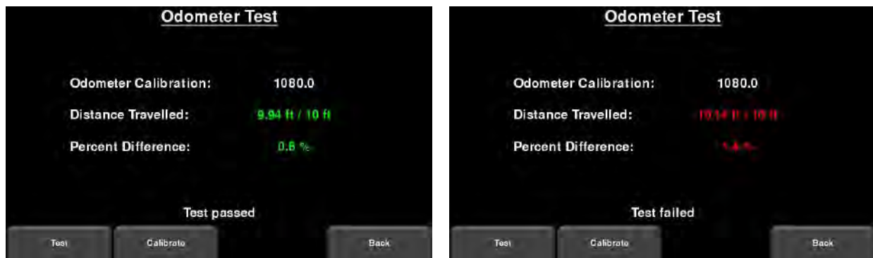
Figure 4-18: Odometer Test passed on left, failed on the right
