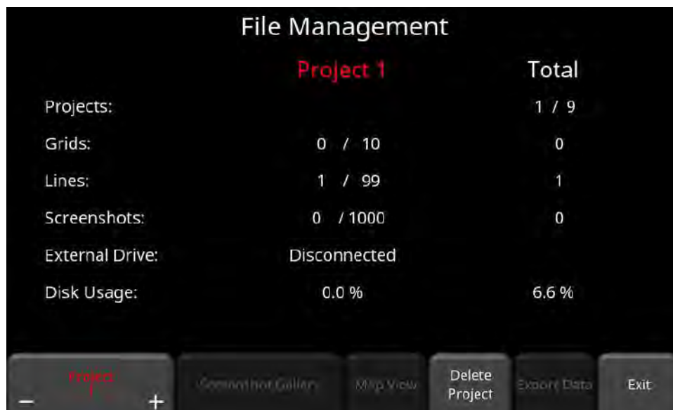
Figure 4-25: File Management displays the lines, grids and screenshots for a given project in the middle column. The right column displays the total for each that are saved on the system.
