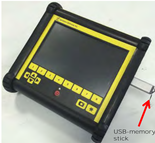
Figure 11-1: Insert a USB memory stick into the USB port on the Display Unit to export data.
