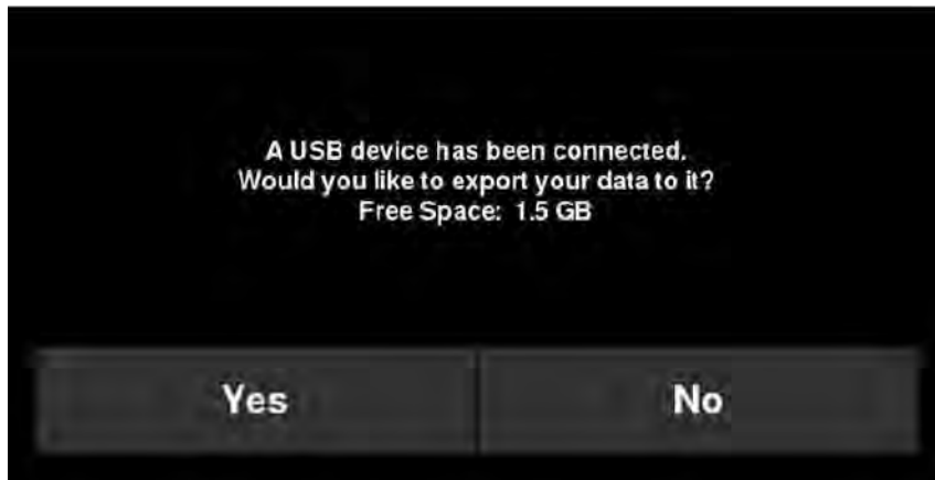
Figure 11-2: When a USB drive is connected to the Display Unit, a message opens asking if you would like to export all your data to it. Select Yes to transfer immediately. If you select No , you can export the data later by going to the Setup > File Management menu option.
