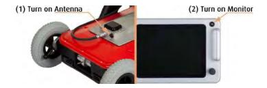
To turn the antenna and monitor off, first select **QUIT** from the **Main Menu** on the monitor, confirm the action by selecting **YES** then push the power button on the monitor and release quickly. The red light will then stop blinking and the unit will also emit a click when turning off.
