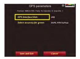
Select the **USB** option to use positioning information acquired via an external USB GPS unit. Once this option is selected, the **Select accuracy for green** option will appear.
