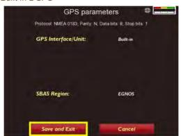
When the Built-in option is selected, the differential correction signal can be received in certain regions enabling better accuracy for the positioned GPS markers. Select the correct region for your area.
