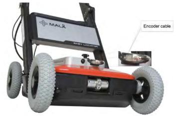
**Note:** The precision of the encoder wheel depends on several factors, such as; the condition of measurement surface, the pressure applied on the wheel and possible wear.
