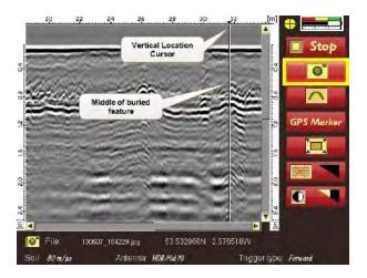
**Tip:** The last signatures can be retained on the screen by lifting the back wheels when moving theMALÅ Easy Locator HDR in position for the next scan. In this way, a comparison between the different scans can be made directly on the screen. This can only be acheived if the GPR profiles are relatively short, as the space on the screen is limited.
