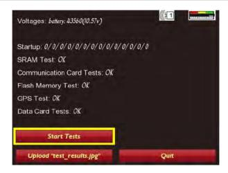
Press the **push-turn knob** with the **Start Tests** button selected to commence the testing. Each item of hardware will be tested sequentially with the results of each tested displayed on the screen and written to a file. Rotate the knob to select the **Quit** button and press to exit this screen.
