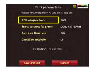
Select the **COM** option to enable positioning information to be acquired via an external GPS unit, such as the RTK survey grade GPS antenna, connected to the **COM port**. Once this option is selected, the **Com port Baud rate** and **Checksum validation** options will appear in the **GPS Parameters** acreen.
