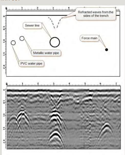
The concrete sewer line in the middle is large enough to leave a signature from both the top and the bottom of the pipe. A close look also shows that the radius of the signature is larger compared to the water pipes to the left. This indicates that the object has a larger diameter.
