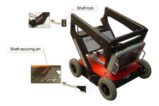
**Tip:** Changing antennas or otherwise dismounting the shaft is best accomplished with the foldable shaft in the extended up-right position. Simply insert the shafts with monitor and battery box attached into the slots on the antenna and secure with the **Shaft securing pins**.
