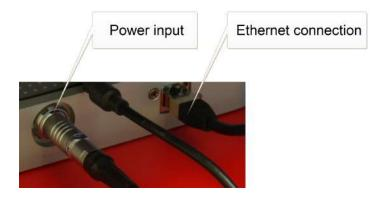
**Note:** The power cable to the rear of the antenna is connected to the battery pack on the RTC, see Battery section below for more information.
