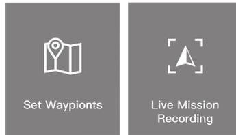
Waypoint flights can be planned in of two ways: Set Waypoints and Live Mission Recording. Use Set Waypoints to create a route by adding editable waypoints on the map. Use Live Mission Recording to create a route by adding waypoints and editing the target in photos captured along the route.
