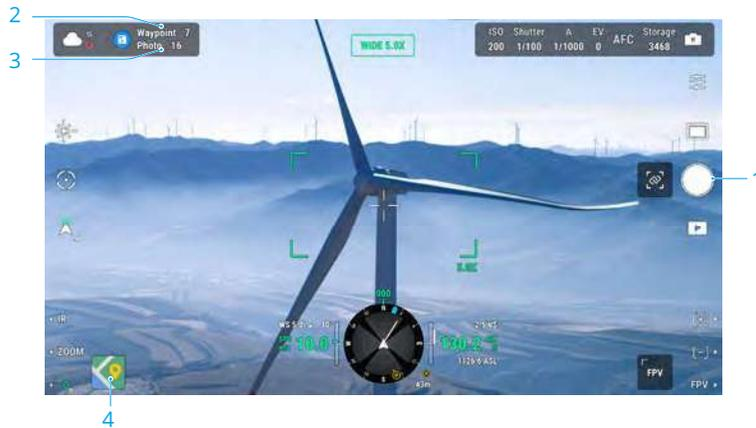
1. Control the gimbal, adjust the camera zoom and aim at the target, and tap to capture a photo directly or press the C1 on the remote controller to set a waypoint. The waypoint and photo quantity will increase accordingly.
