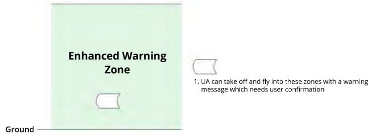
Warning Zones: warning message will be shown to user when the drone reaches the edge of the zones.
