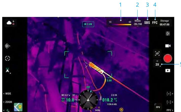
1. **Palette/Isotherm:** displays the highest and lowest temperature measurement values of the current view. Tap to choose between different infrared temperature measurement palettes, or enable the isotherm to set temperature measurement intervals. Note that if the measured area exceeds the maximum or minimum temperature measurement values of the current view, the setting will not take effect.
