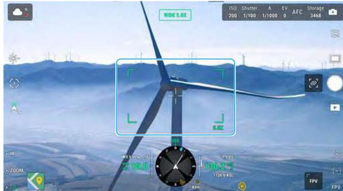
**Zoom Frame:** After switching to a wide-angle camera as the main view, the zoom frame will display the field of view and camera zoom rate.
