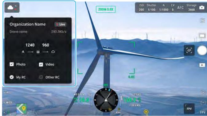
26. **Mission Flight Control/Status:** displays the progress of a mission flight in gimbal camera view. Tap the Pause/Resume button to pause/resume the task, and tap the panel to view the mission flight name and actions.
